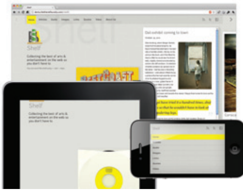
FIG 4.28: Jon Hicks' responsive "Shelf" theme for WordPress and Tumblr ( http://bkaprt.com/rwd/41/ ) has a beautifully flexible layout, but contains fixed-width containers for different kinds of entries. (Love that horizontal scrolling!)
